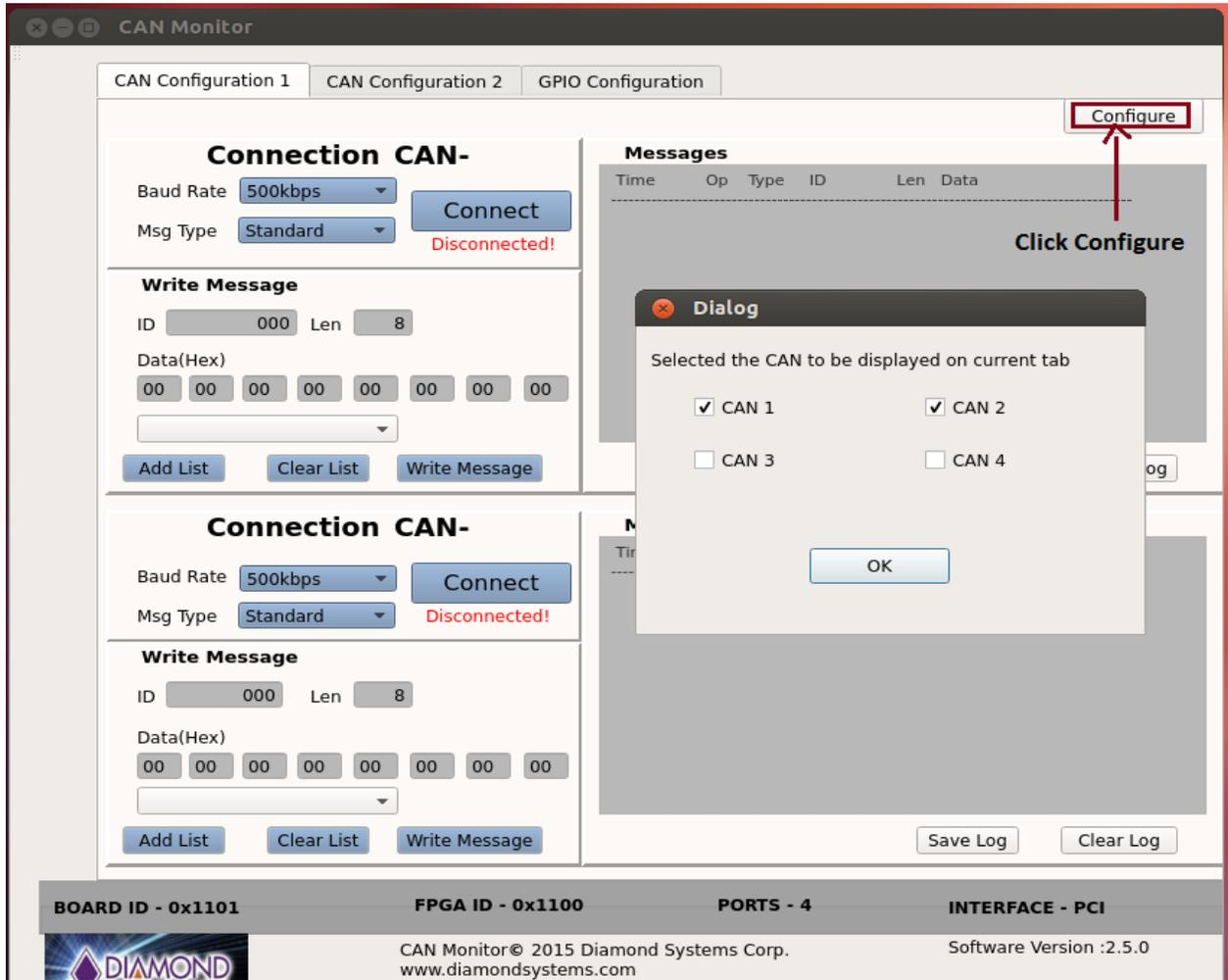
Initially CAN numbers will be empty on each tab. After configuring the CAN ports, the selected CAN # number will be displayed.
