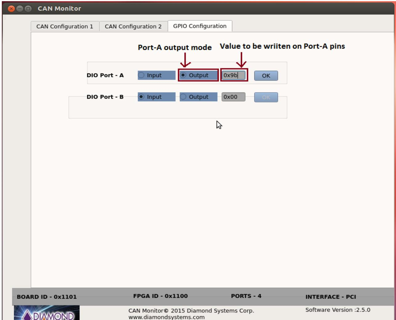
Similarly, Port-B can be configured as either an input or output port.
