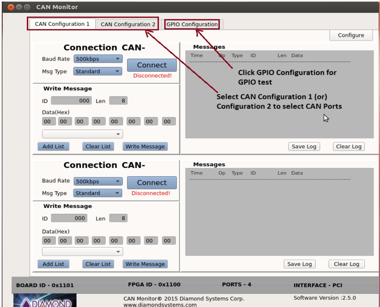
A Pop-up window will appear by clicking on the “Configure” button when selecting any two CAN ports for each tab. After selecting, click on OK.
